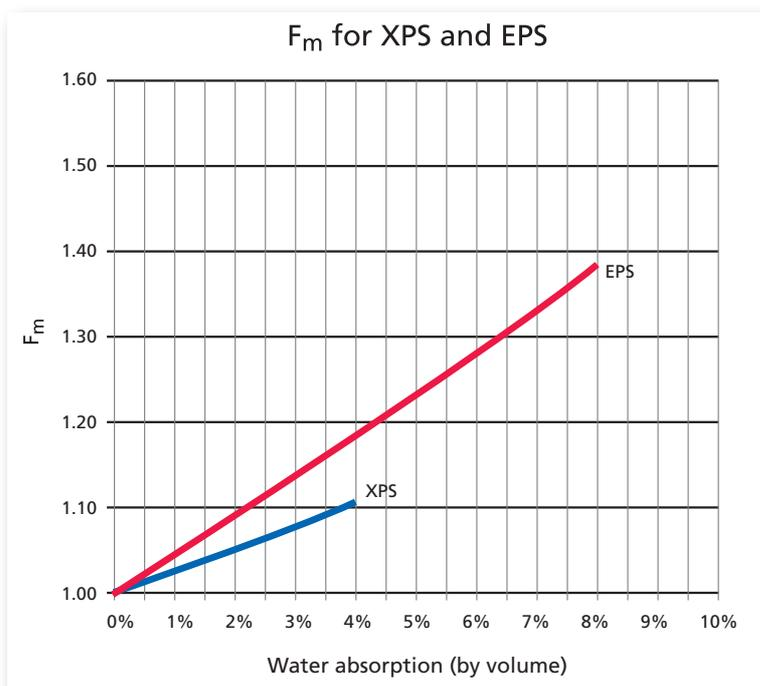
Figure 1:  $F_m$  for XPS and EPS. Plots terminated at maximum permitted absorption level for XPS and EPS.
