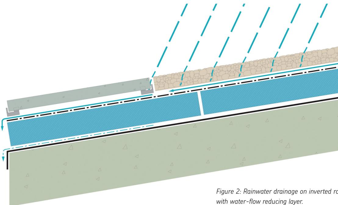
Figure 2: Rainwater drainage on inverted roofs with water-flow reducing layer.
